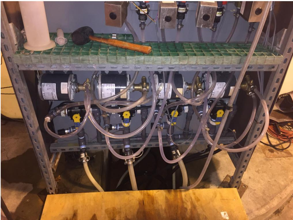
Left pump only was used to pump water from storage/aeration tanks to top of Filter 1.
