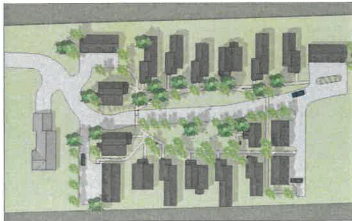
The cottages can be arranged as a common courtyard with parking at the edges and a pedestrian center.
