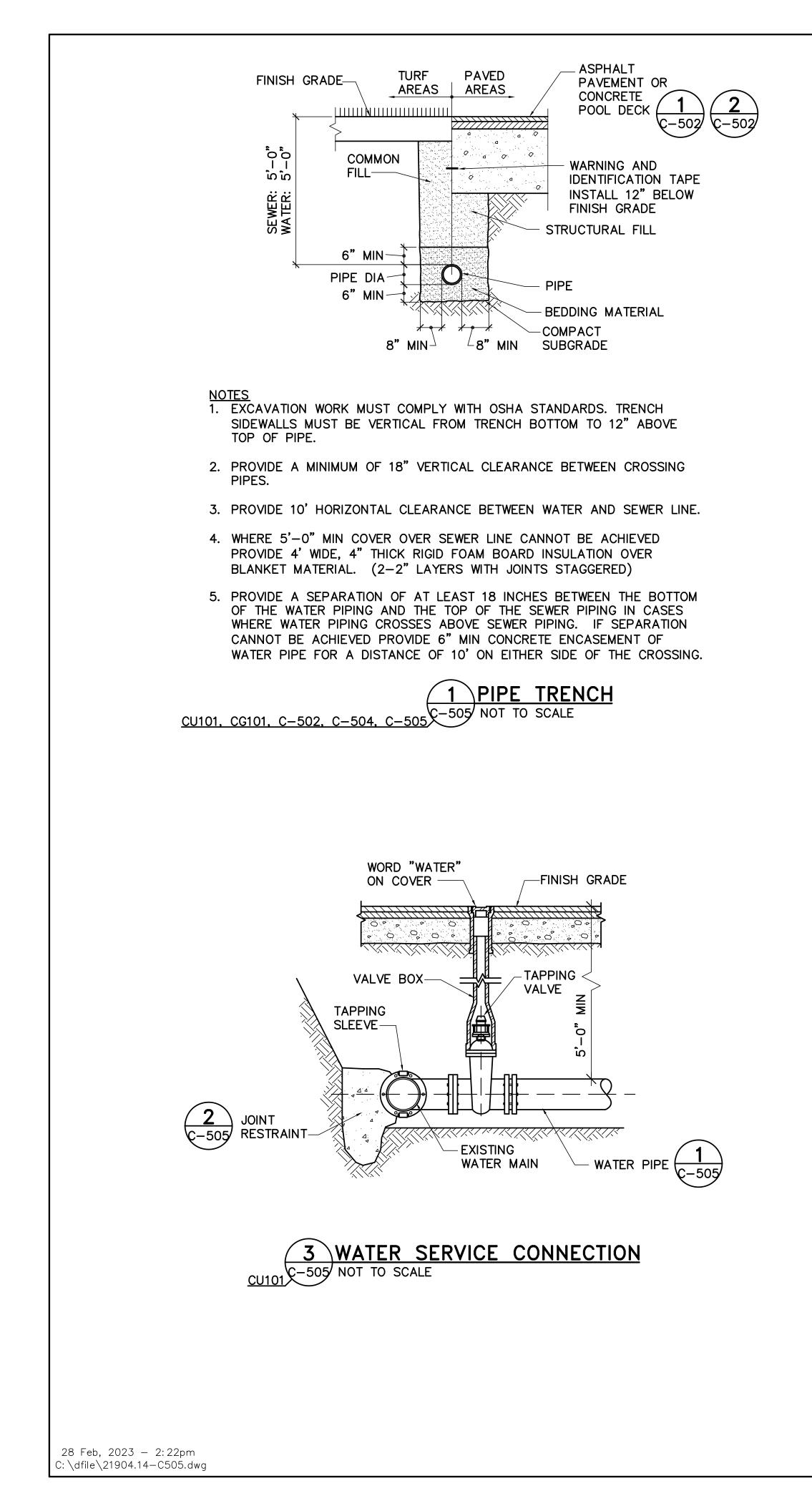
NOTES 1. PROVIDE JOINT RESTRAINT FOR TEES, BENDS, AND PLUGS. FOR DUCTILE IRON PIPE PROVIDE CONCRETE THRUST BLOCKS AND WEDGE-ACTION TYPE RETAINER GLANDS. FOR POLYETHYLENE PIPE PROVIDE CONCRETE THRUST BLOCKS.
