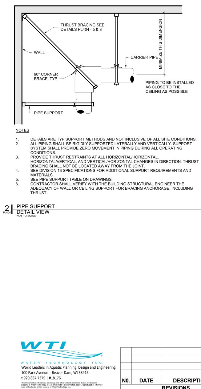
5 PIPE THRUST BRACING DETAIL VIEW
