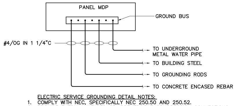
2. PROVIDE THERMAL WELDED OR IRREVERSIBLE COMPRESSION CONNECTIONS.
