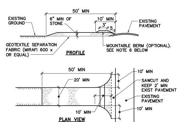
1. PROVIDE 2 TO 3 INCH STONE, RECLAIMED STONE, OR RECYCLED CONCRETE EQUIVALENT.
