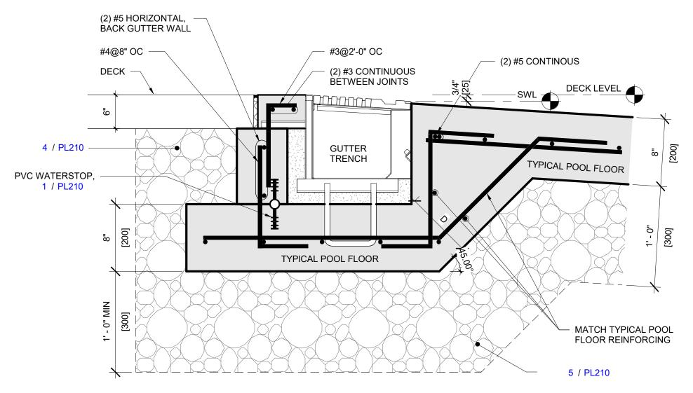
3 REINFORCING - ZERO DEPTH GUTTER SECTION VIEW
