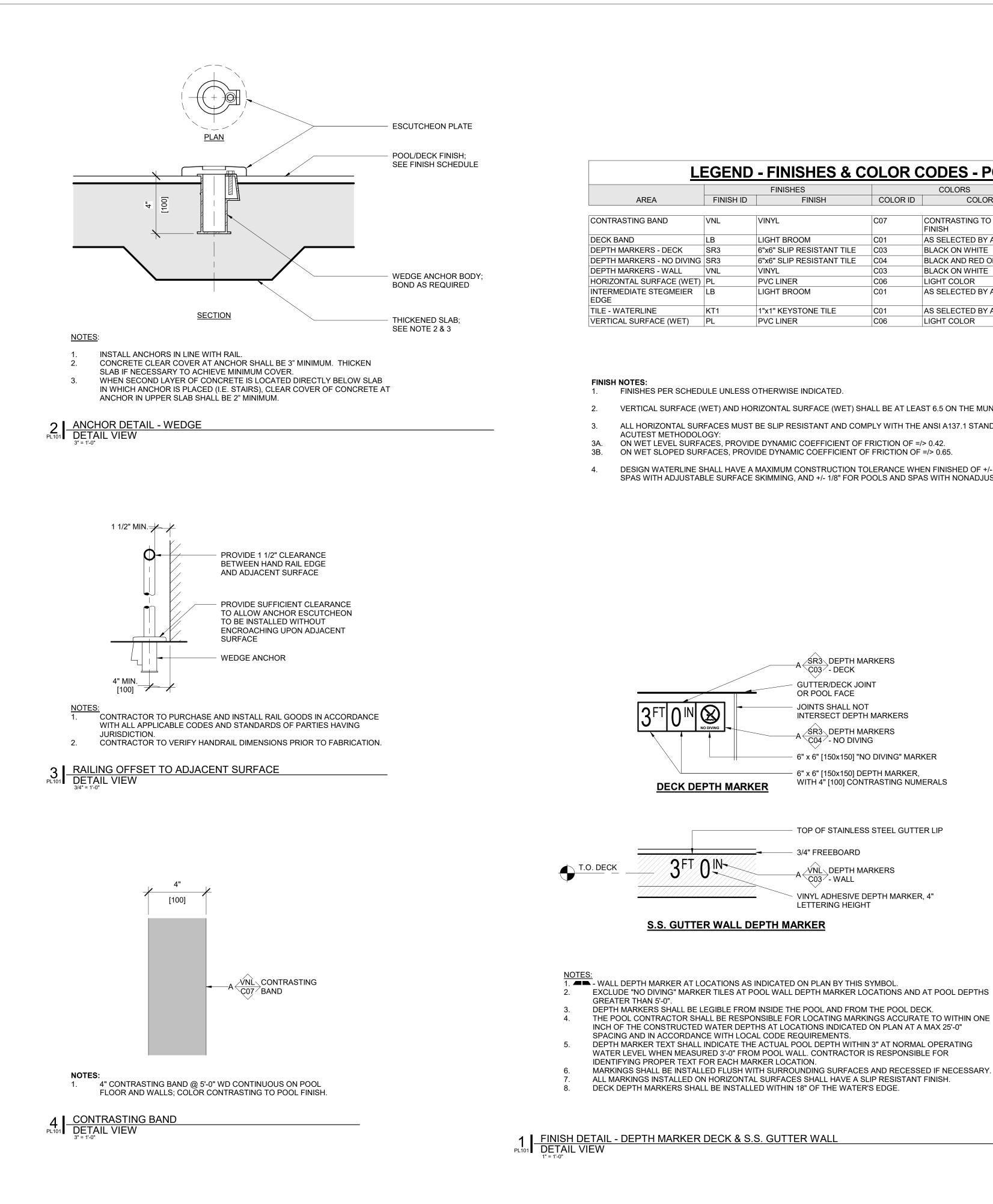
INCH OF THE CONSTRUCTED WATER DEPTHS AT LOCATIONS INDICATED ON PLAN AT A MAX 25'-0" SPACING AND IN ACCORDANCE WITH LOCAL CODE REQUIREMENTS.
