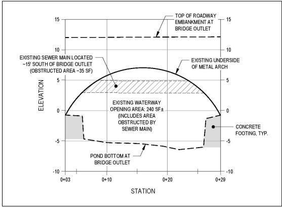
Figure 16 – Existing bridge outlet cross-section
