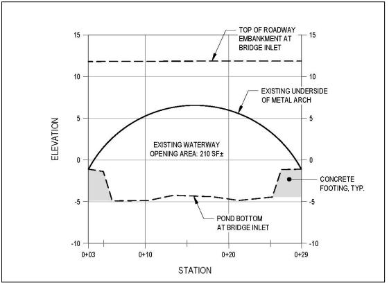
*Figure 15 – Existing bridge inlet cross-section*
