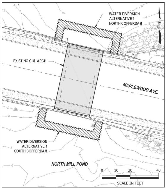
Figure 34 – Water Diversion Alternative 1 Schematic Plan
