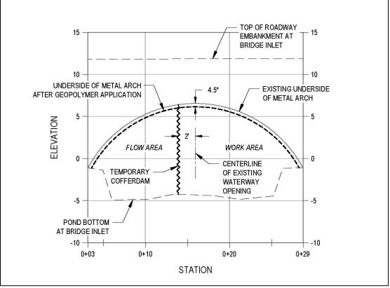
Figure 46 – Water Diversion Alternative 3 Bridge Inlet Cross-Section
