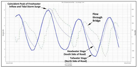
Figure 26 – 100-year stage and flow hydrographs calculated at the bridge for Bridge Rehabilitation Alternative 1
