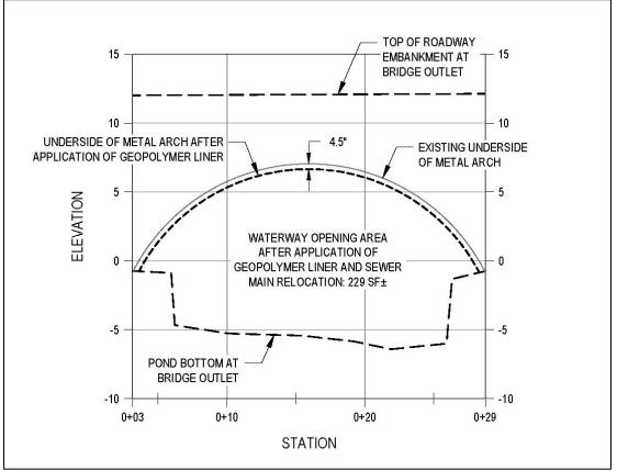
Figure 30 - Bridge Rehabilitation Alternative 3 outlet cross-section
