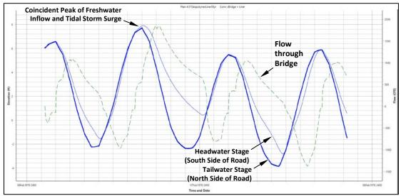
Figure 25 – 50-year stage and flow hydrographs calculated at the bridge for Bridge Rehabilitation Alternative 1
