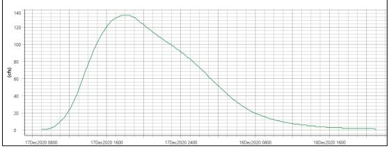
Figure 38 – Assumed freshwater inflow hydrograph for Water Diversion Alternatives 2 through 4
