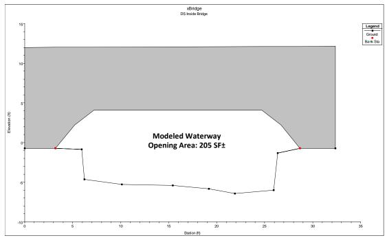
Figure 18 – Existing bridge outlet cross-section as modeled to account for sewer main obstruction
