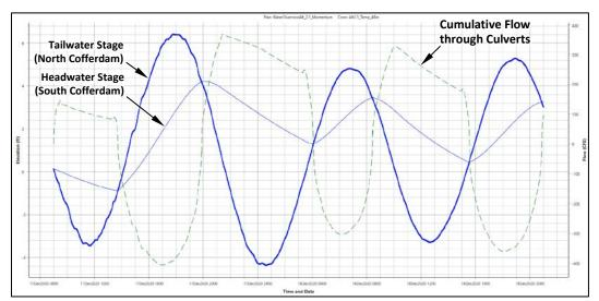
Figure 41 – Stage and flow hydrographs calculated at the bridge for Water Diversion Alternative 2.1
