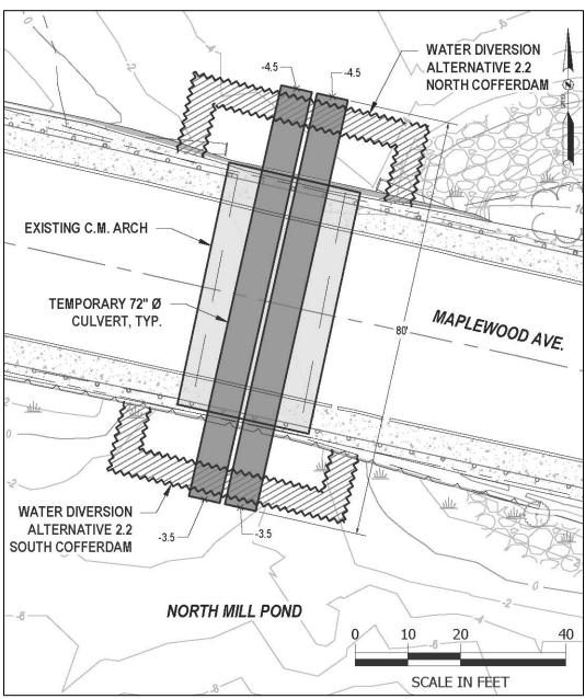
Figure 43 – Water Diversion Alternative 2.2 Schematic Plan
