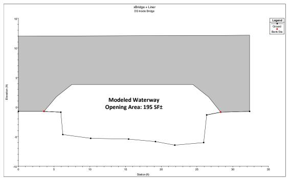
Figure 24 – Bridge Rehabilitation Alternative 1 bridge outlet cross-section as modeled to account for geopolymer liner and sewer main obstructions
