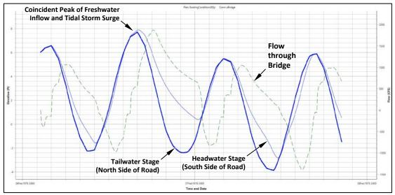
Figure 21 – Existing conditions 50-year stage and flow hydrographs calculated at the bridge
