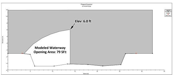
Figure 47 - Bridge inlet cross-section as coded in the hydraulic model for Water Diversion Alternative 3
