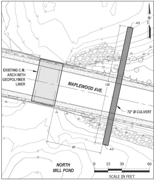
Figure 29 – Bridge Rehabilitation Alternative 2.3 schematic plan
