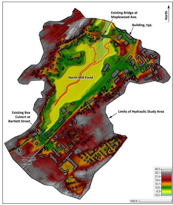
Figure 5 – Existing conditions digital elevation model (DEM) of the hydraulic study area showing areas field surveyed by Doucet Survey, LLC outlined in red and areas field surveyed by Headwaters Consulting, LLC outlined in blue
