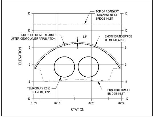
Figure 44 – Water Diversion Alternative 2.2 Bridge Inlet Cross-Section
