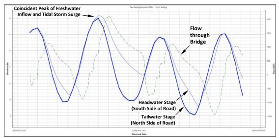
Figure 22 – Existing conditions 100-year stage and flow hydrographs calculated at the bridge
