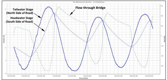
Figure 48 – Stage and flow hydrographs calculated at the bridge for Water Diversion Alternative 3
