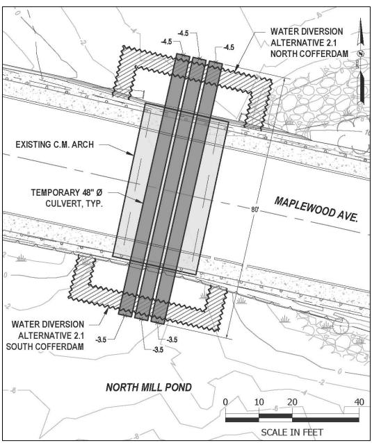
Figure 39 – Water Diversion Alternative 2.1 Schematic Plan
