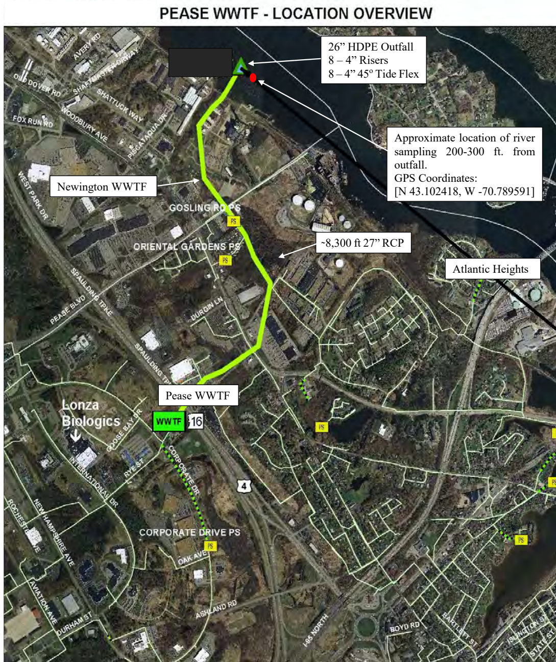
Figure 1: Overview map of WWTF locations, combined outfall, and Piscataqua River sampling location.
