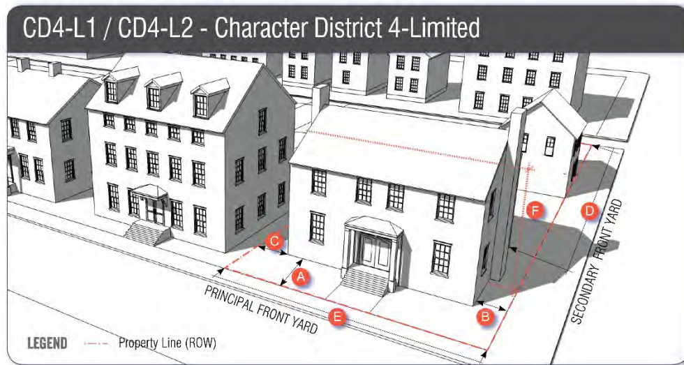
FIGURE 10.5A41.10A DEVELOPMENT STANDARDS CHARACTER DISTRICT 4—LIMITED (CD4-L1/CD4-L2)
