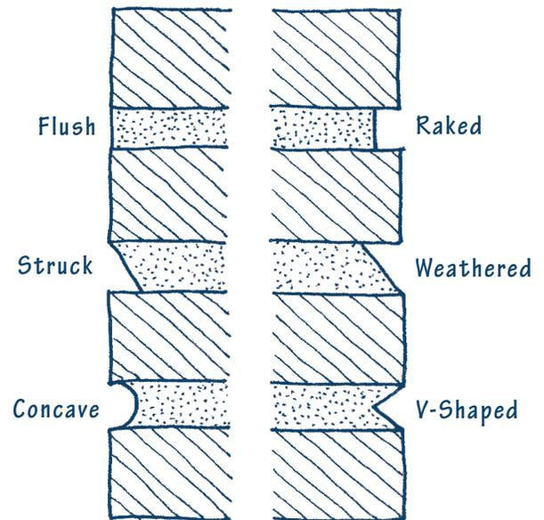
There are numerous mortar joint profile types, or shapes, with each producing different shadow lines and highlights. When repointing an area of masonry, it is important to tool the mortar to match the existing joint profile for a consistent appearance.
