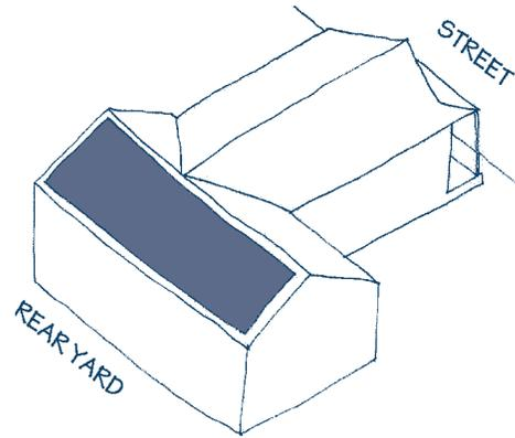
Placement of roof-mounted equipment, solar collectors, wind turbines, skylights and roof hatches is encouraged facing a rear yard wherever possible. If it is not possible, placement as far back on a side roof slope as possible is preferred.
