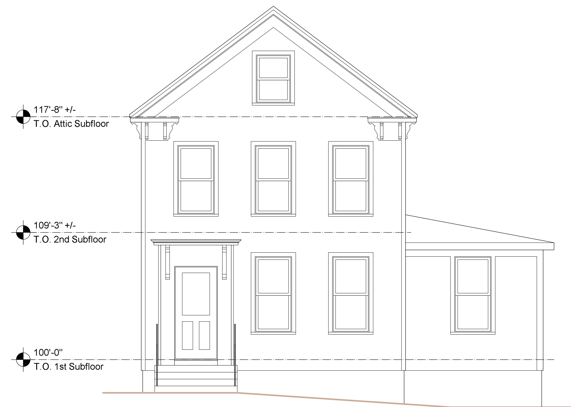
EXISTING FRONT ELEVATION
