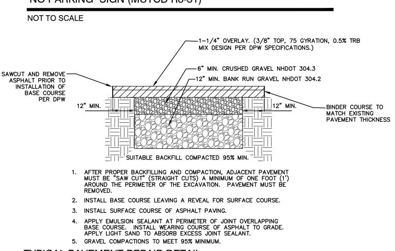
TYPICAL PAVEMENT REPAIR DETAIL
