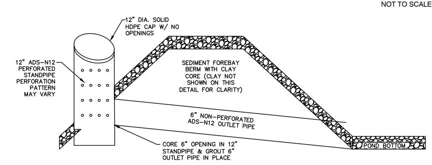
PERFORATED SEDIMENT FOREBAY STANDPIPE
