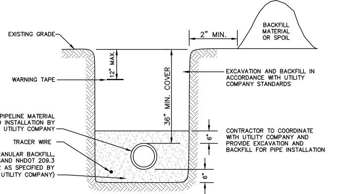
GAS PIPELINE MATERIAL AND INSTALLATION BY GRANULAR BACKFILL SAND NHDOT 209.3 (OR AS SPECIFIED BY UTILITY COMPANY) -
