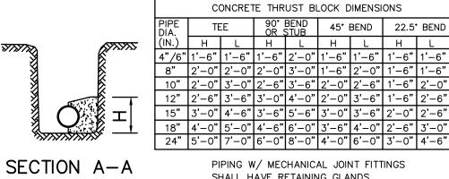
90° BEND | 45° BEND | 22.5° BEND OR AS REQUIRED SECTION B-B
