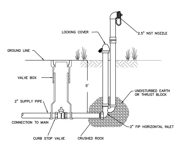
POST HYDRANTS SHALL BE NON-FREEZING, SELF DRAINING TYPE WITH A 5' BURY. THESE HYDRANTS WILL BE FURNISHED WITH A 2" FIP HORIZONTAL INLET, A NON-TURNING OPERATING ROD, AND SHALL OPEN LEFT. BRONZE OPERATING MECHANISM AND ALUMINUM PLUNGER. DESIGN, AND BE SERVICABLE FROM ABOVE GRADE WITH NO DIGGING. THE OUTLET SHALL ALSO BE BRONZE AND BE 2-1/2" NST. HYDRANTS SHALL BE LOCKABLE TO PREVENT UNAUTHORIZED USE AS MANUFACTURED BY KUPFERLE FOUNDRY CO., ST. LOUIS, MO, OR
