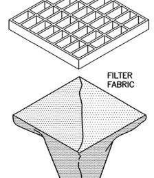
1) INLET BASKETS SHALL BE INSTALLED IMMEDIATELY AFTER CATCH BASIN CONSTRUCTION IS COMPLETE AND SHALL REMAIN IN PLACE AND BE MAINTAINED UNTIL PAVEMENT BINDER COURSE IS FILTER FABRIC SHALL BE PUSHED DOWN AND ORMED TO THE SHAPE OF THE BASKET. THE SHEET
