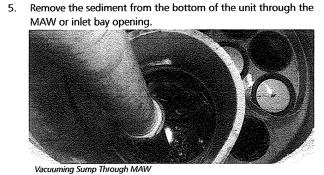
For larger diameter Jellyfish Filter manholes (≥8-ft) and some vaults complete sediment removal may be facilitated by removing a cartridge lid from an empty receptacle and inserting a jetting wand (not a vacuum wand) through the receptacle. Use the sprayer to rinse loosened sediment toward the vacuum hose in the MAW opening, being careful not to damage the
