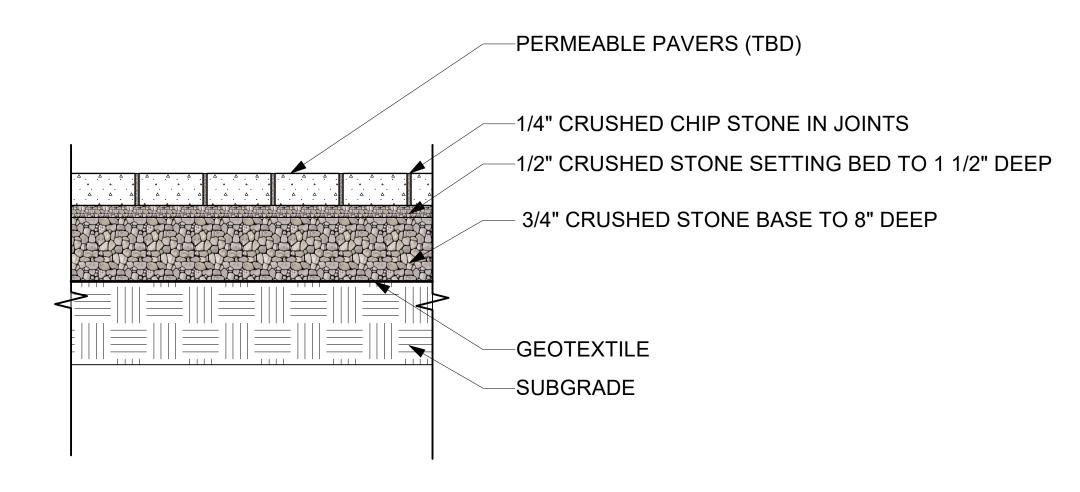
POROUS SIDEWALK DETAIL SCALE: 1" = 1'-0" L-3
