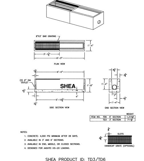
$\overline{\begin{array}{c} AA \\ C6 \end{array}}$  STRIP DRAIN
