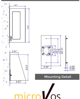
Ligman's micro Variable Optical System provides the ability to interchange, mix & rotate optics to provide specific light distributions for optimized spacing and uniformity.
