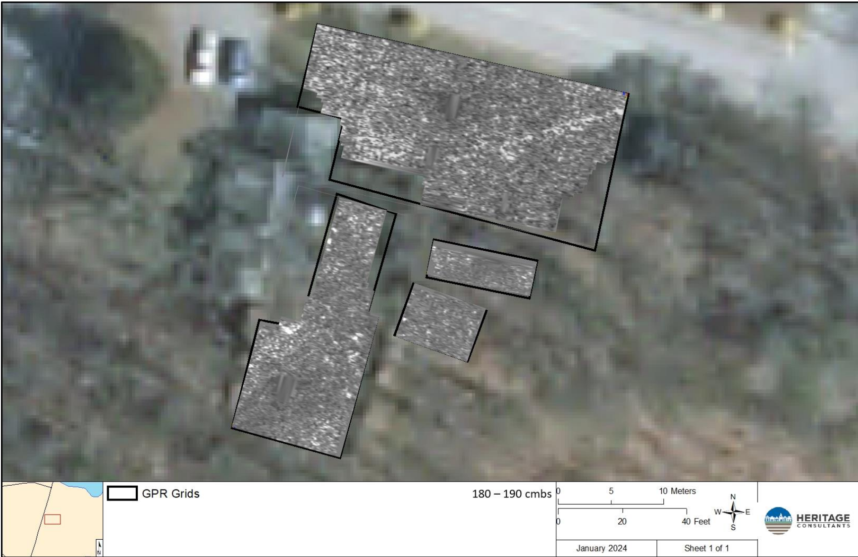
Figure 30: GPR amplitude map of Survey Grids 1-4, with approximate depth indicated.
