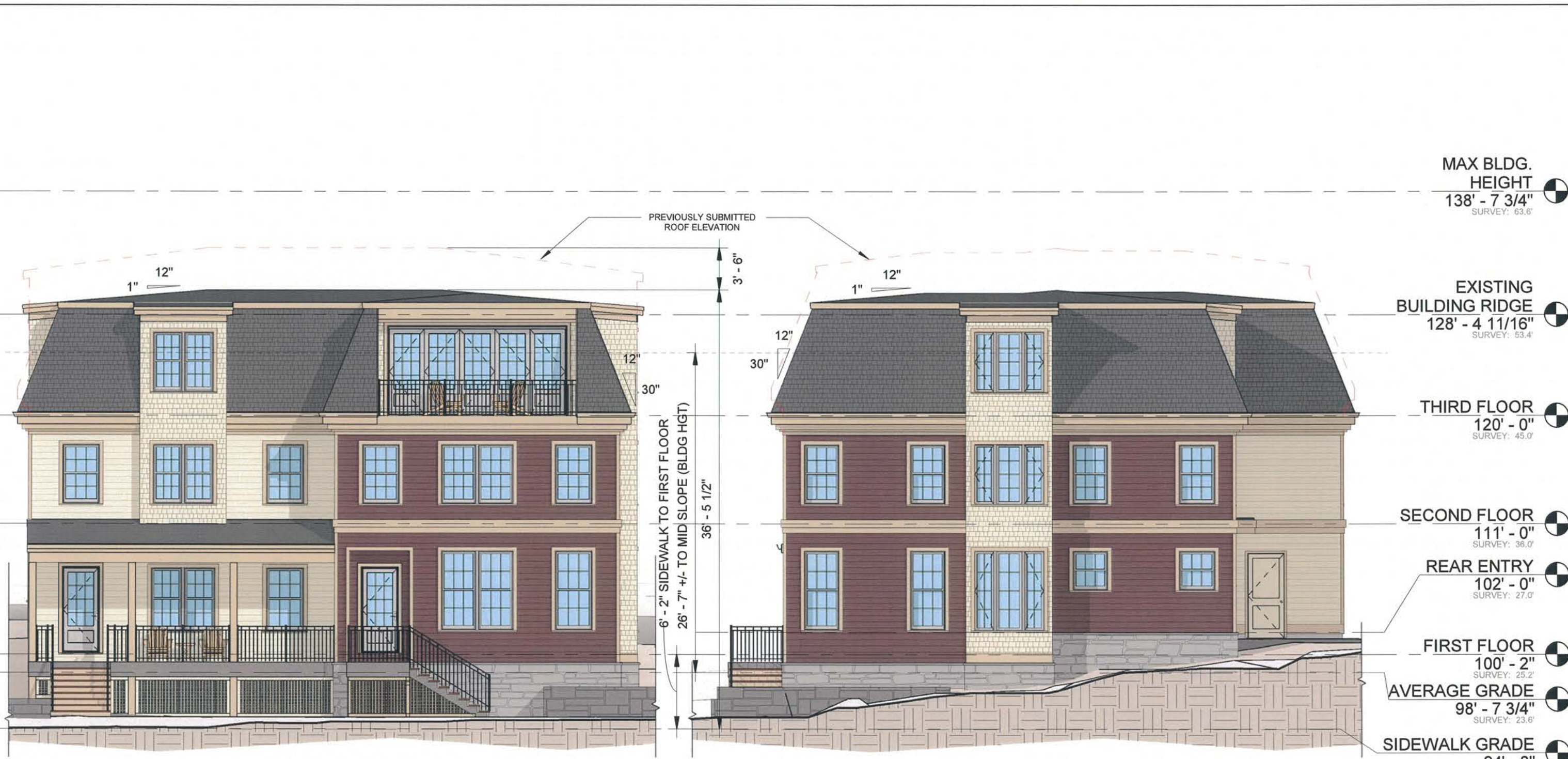
1 NORTH-WEST ELEVATION - HANOVER STREET 1/8" = 1'-0"
