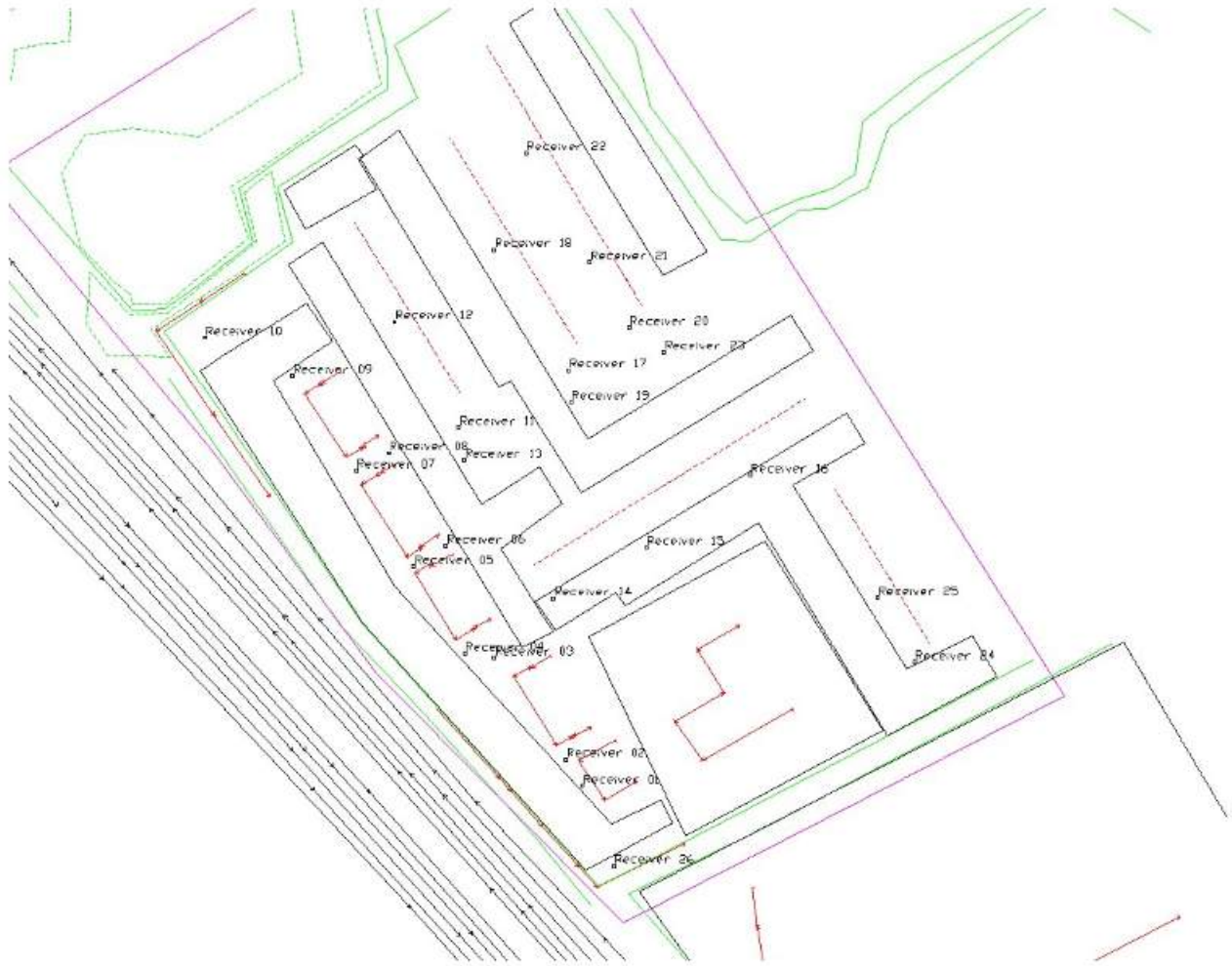
Figure 3. Receivers, numbered 1 through 26, included in the noise analysis.
