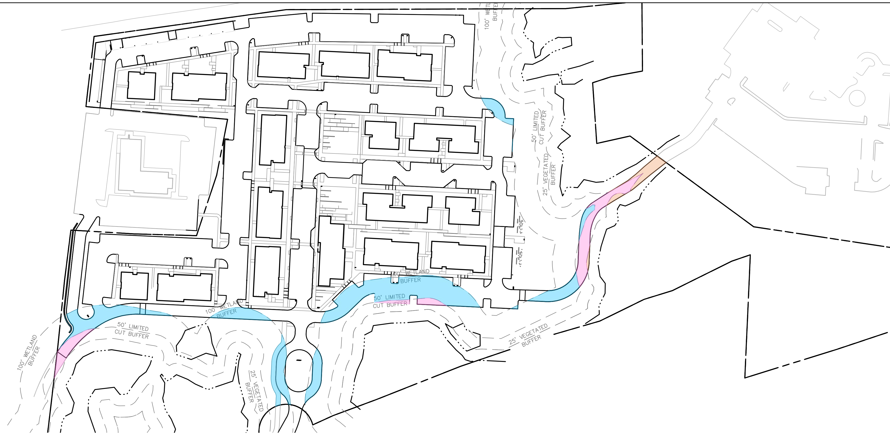
PROPOSED WETLAND BUFFER IMPERVIOUS SURFACE SCALE 1" = 100'
