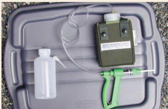
Hollow stem injection tools.
