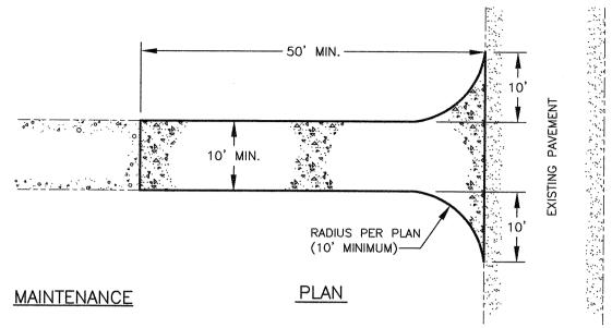
1) MUD AND SOIL PARTICLES WILL EVENTUALLY CLOG THE VOIDS IN THE GRAVEL AND THE EFFECTIVENESS OF THE GRAVEL PAD WILL NOT BE SATISFACTORY. WHEN THIS OCCURS, THE PAD SHOULD BE TOP DRESSED WITH NEW STONE. COMPLETE REPLACEMENT OF THE PAD MAY BE NECESSARY WHEN THE PAD BECOMES COMPLETELY CLOGGED.
