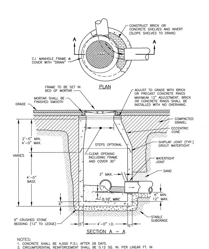
4. EACH CASTING TO HAVE LIFTING HOLES CAST IN. DRAIN MANHOLE DETAIL
