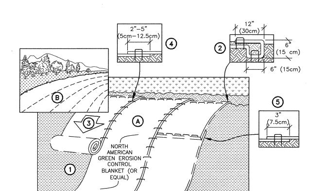
PREPARE SOIL BEFORE INSTALLING ROLLED EROSION CONTROL PRODUCTS (RECP'S), INCLUDING ANY NECESSARY APPLICATION OF LIME, FERTILIZER, AND SEED. NOTE: WHEN USING CELL-O-SEED DO NOT SEED PREPARED AREA. CELL-O-SEED MUST BE INSTALLED WITH PAPER SIDE DOWN.
