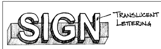
(c) Internally illuminated channel letters.
