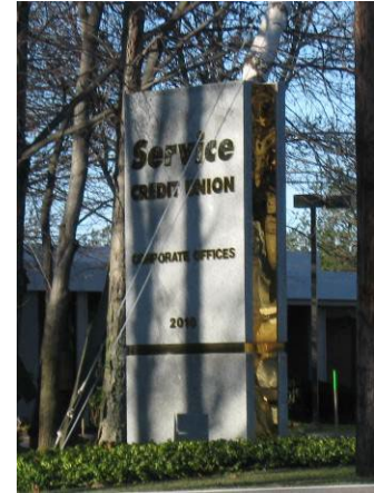
Height of base is greater than one foot – Included in sign area
