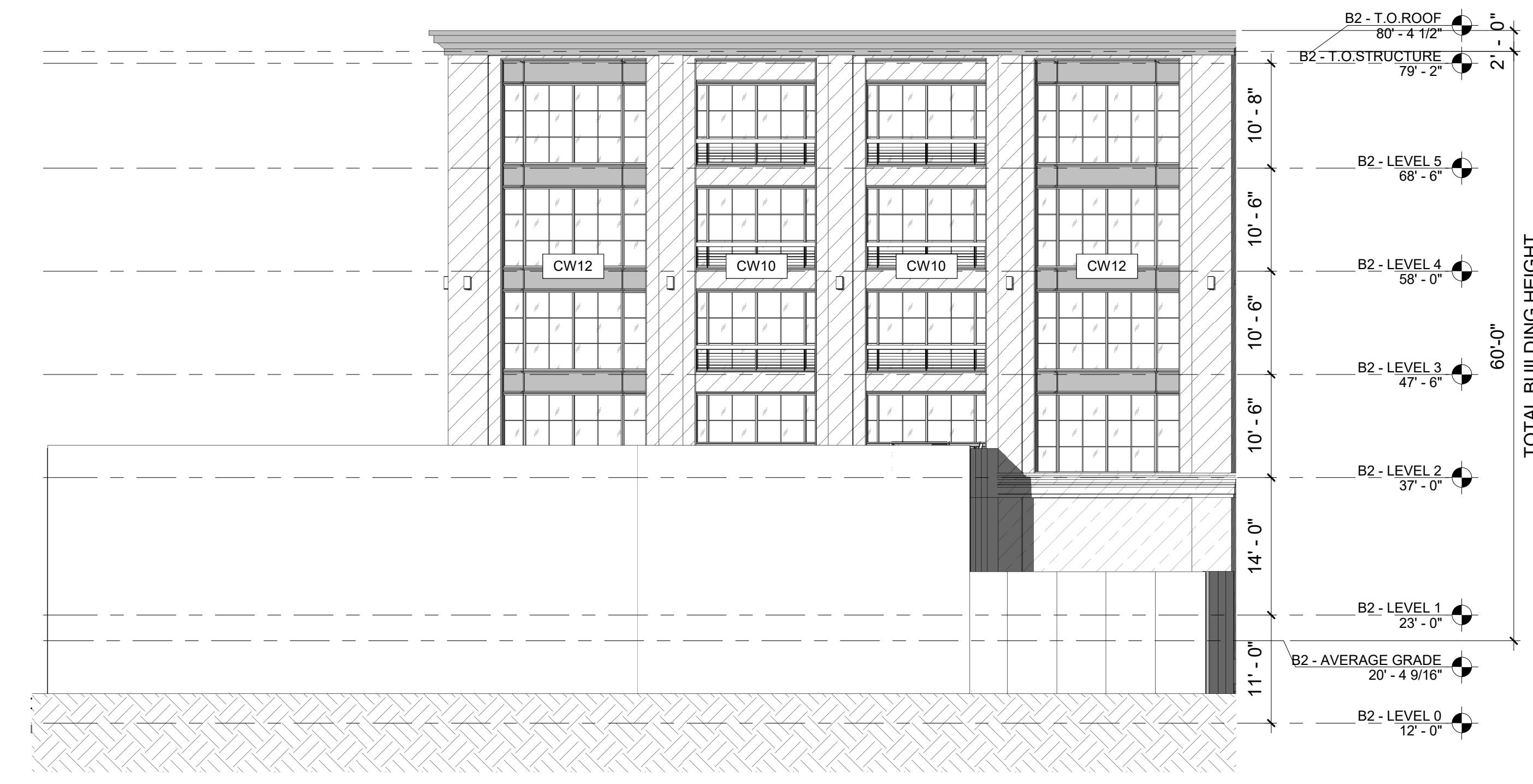
5 B2 - North-West Elevation 3/32" = 1'-0"
