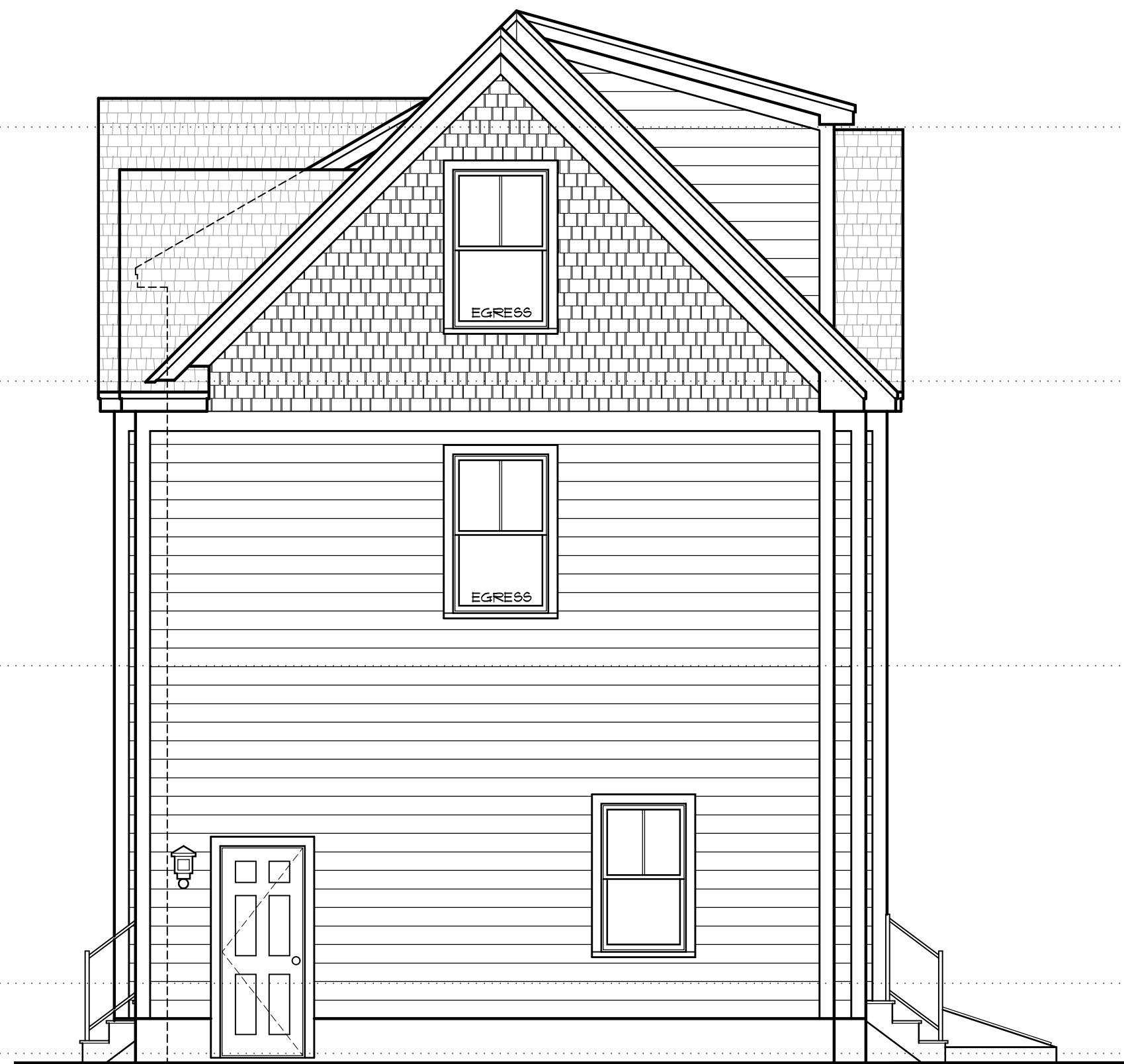
RIGHT SIDE ELEVATION 1/4" = 1'-0"
