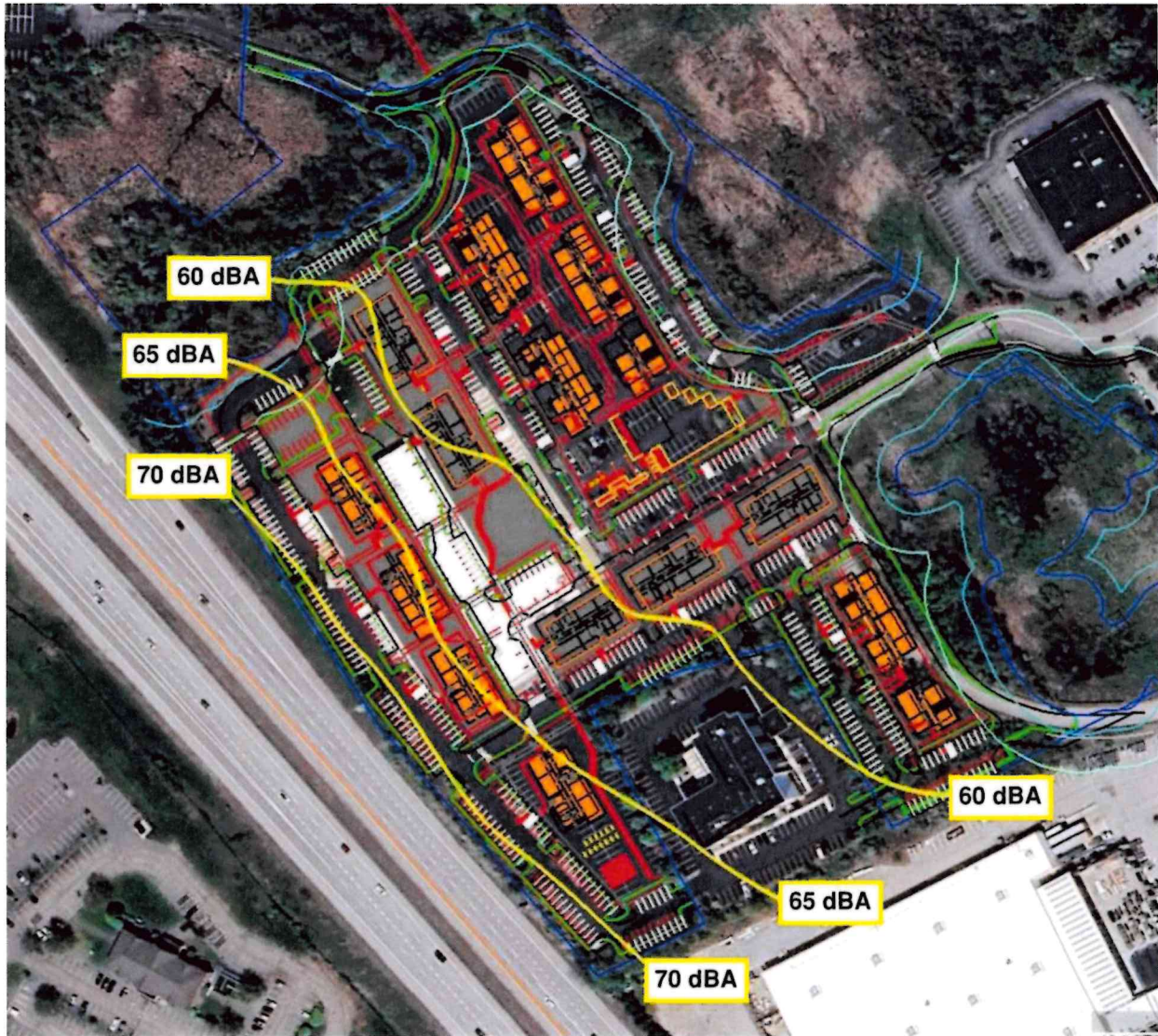
Figure 4. Unadjusted 60, 65, and 70 dBA noise contours (5 ft elevation) overlaid upon the Project site diagram based upon Year 2022 traffic data.
