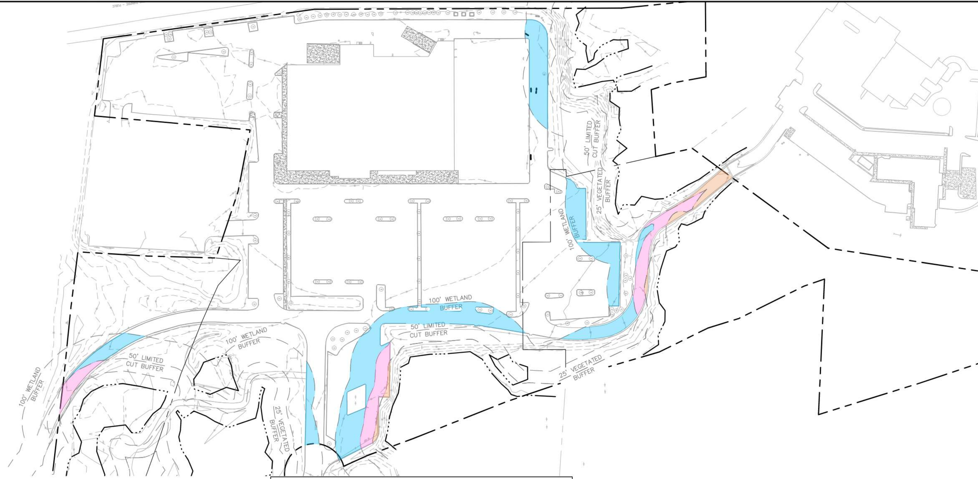
EXISTING WETLAND BUFFER IMPERVIOUS SURFACE SCALE 1" = 100'
