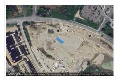
Name: LGBLDG Footprint area: 2.0 acres Axis tracking: Fixed (no rotation) Tilt: 15.0 deg Orientation: 214.0 deg
