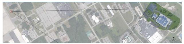
To establish a <u>worst-case scenario</u> baseline, a 15-degree angle for the proposed rooftop system facing 214 degrees (azimuth) was programmed on the rooftops of two buildings. For the proposed carports, four array areas were programmed facing 124 degrees (azimuth) and one carport was programmed facing 214 degrees (azimuth). The project was modeled <u>without</u> local foliage lines and other large buildings between the proposed project and the ATCT in the area programmed.
