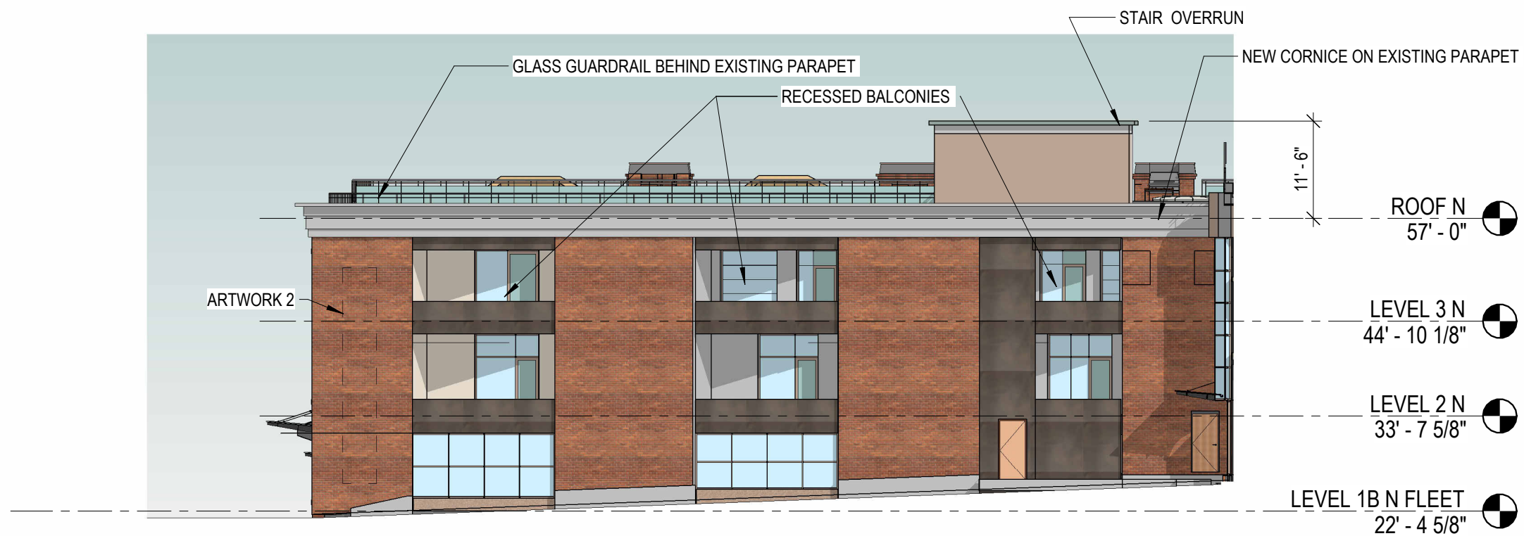
3 SOUTH ELEVATION - SOUTH ALLEY 1/16" = 1'-0"
