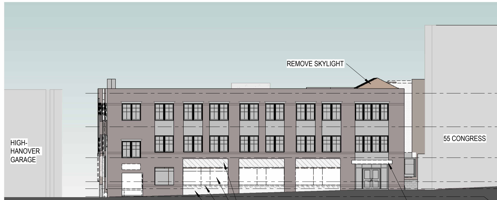
2 WEST ELEVATION - FLEET STREET, EXISTING 1" = 20'-0"
