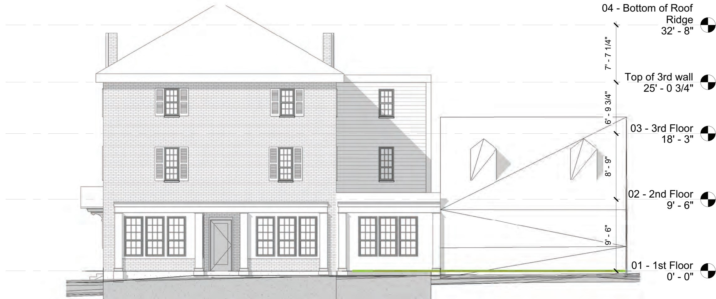
Existing Elevation - North | Scale: 1"=1/8"
