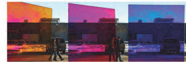
In Transmission (Shown) Yellow ▶ Magenta ▶ Blue In Reflection Gold (straight) Blue (angle)
