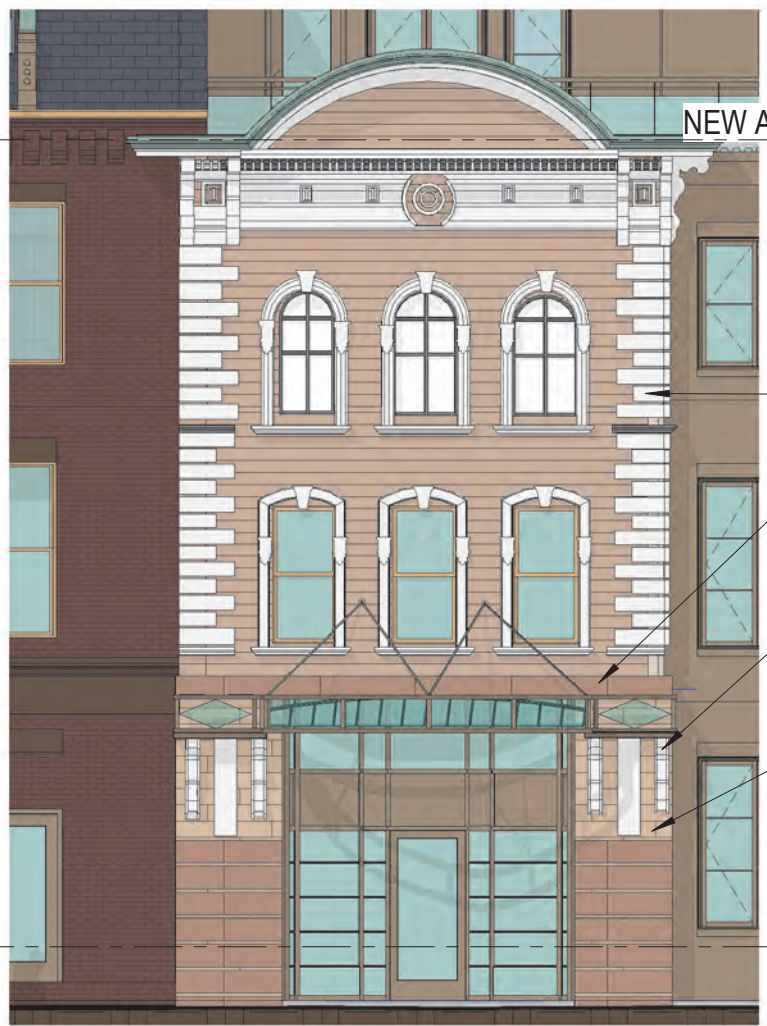
2 PROPOSED ELEVATION - NE - HIGH STREET 1/8" = 1'-0"
