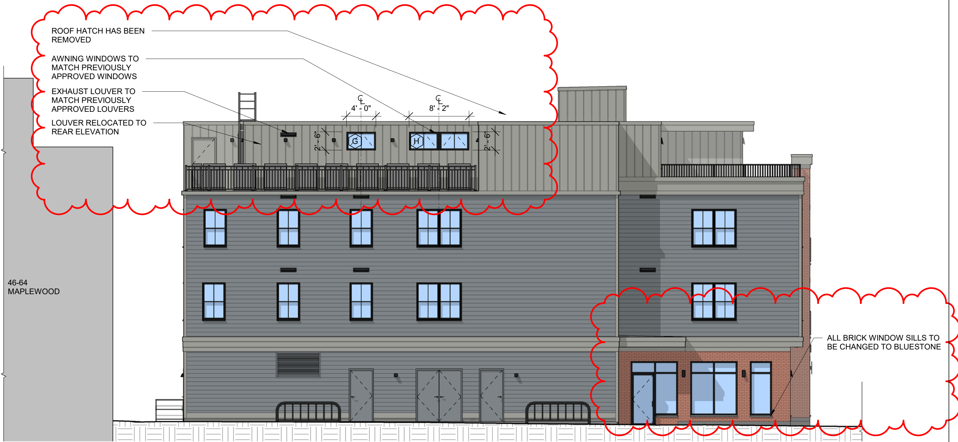
1 EAST ELEVATION (PUBLIC WALKWAY) 1/8" = 1'-0"
