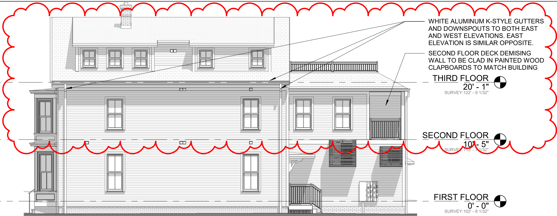
1 WEST ELEVATION (RIGHT SIDE YARD) 1/8" = 1'-0"
