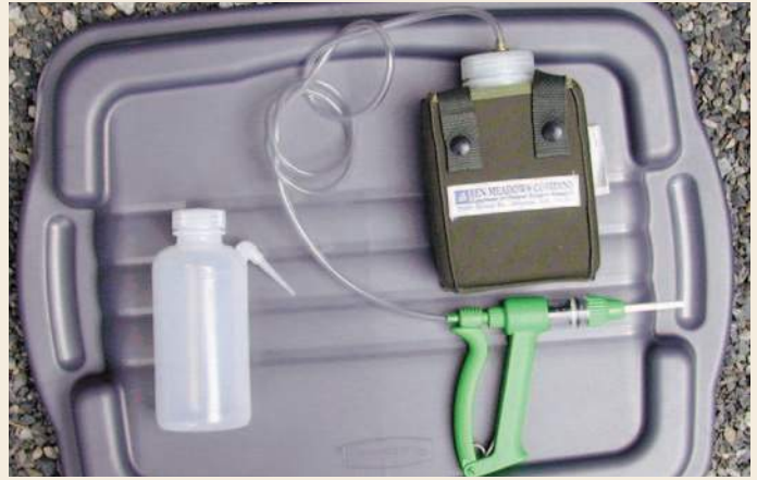
Hollow stem injection tools.
