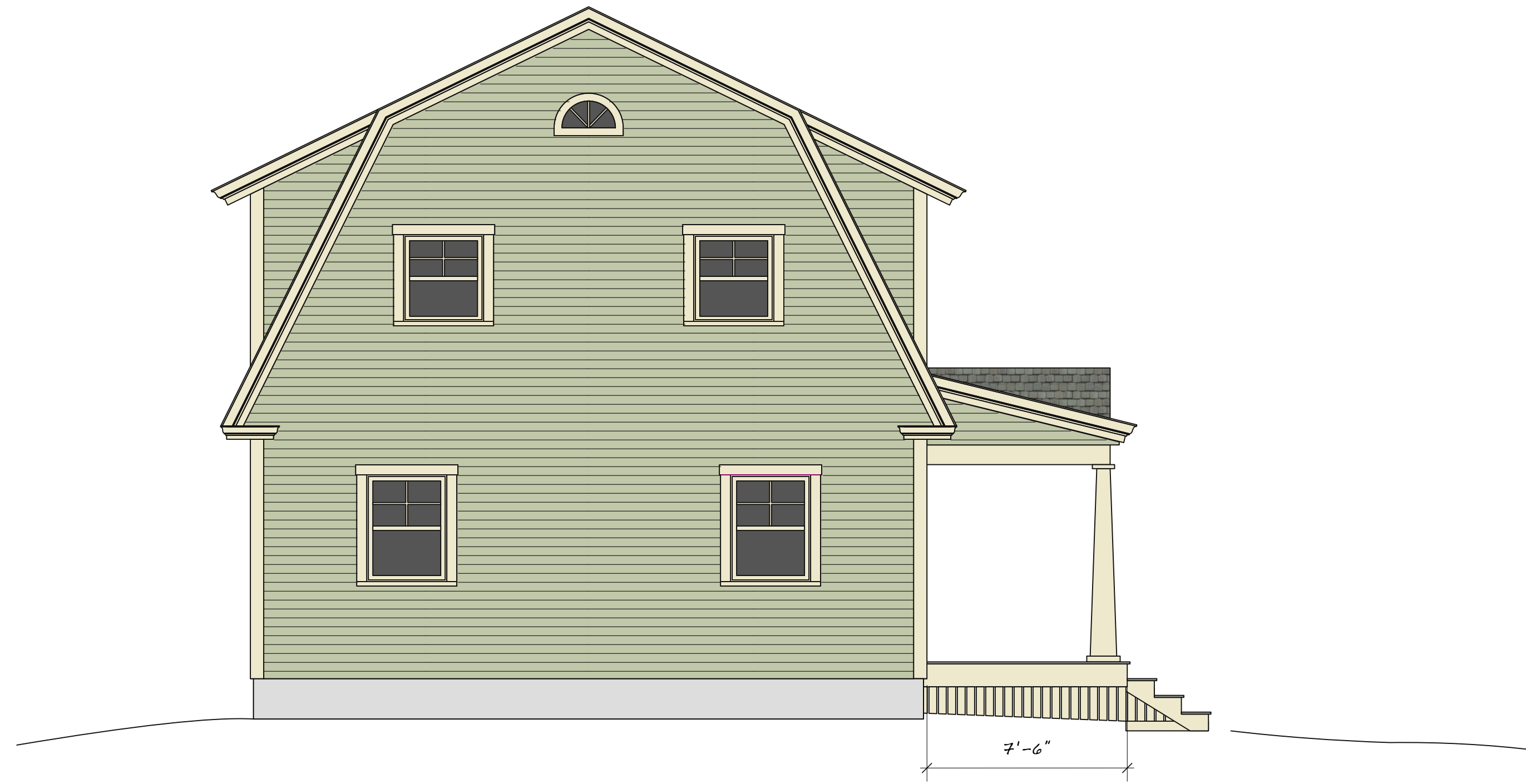
7.0 Side Elevation Scale: 1/4" = 1'-0"
