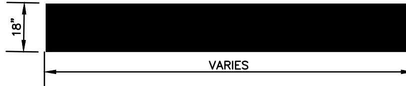
KEYWAY DETAIL FOR CONNECTION TO EXISTING PAVEMENT
