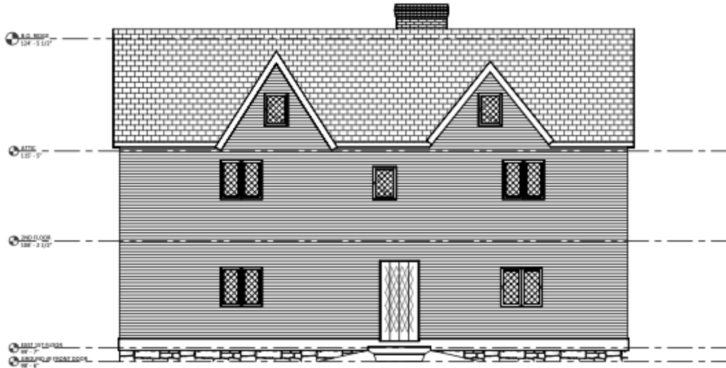
02 EXTERIOR ELEVATION - SOUTH 1/4" = 1'-0"
