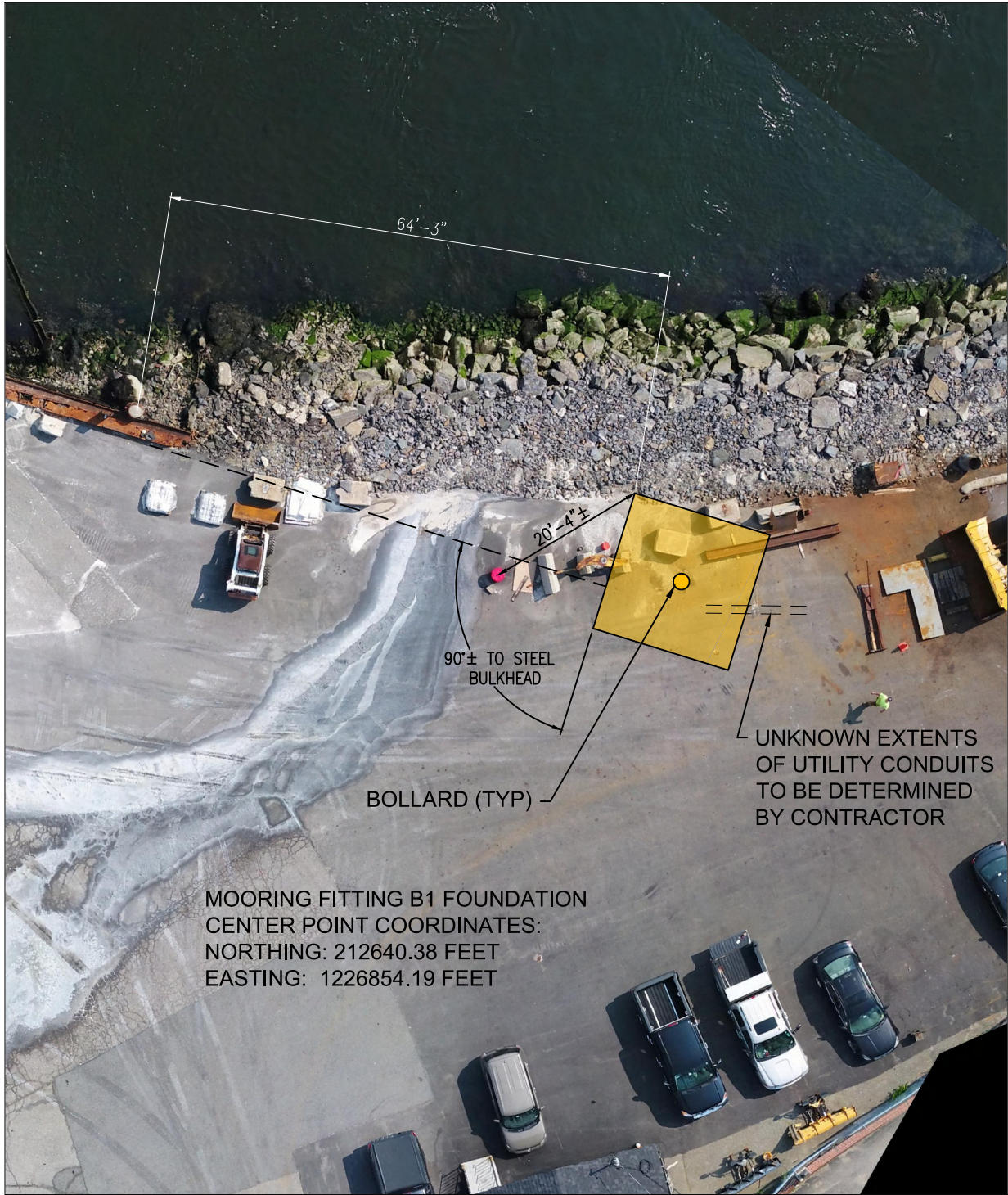
MOORING FITTING B1 LOCATION PLAN SCALE: 1"=10'-0" PLAN NORTH
