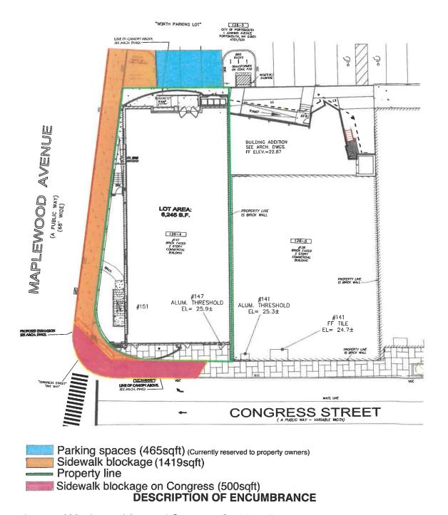
Temporary closure of Maplewood Ave and Congress St sidewalk to excavate structural footings for addition located at 147 Congress Street (blue). Occupy three parking spaces immediately in rear of property for dumpster and loading of construction materials. Rear parking spaces are currently reserved for the property owners from 8am to 8pm.
