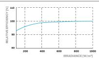
Typical module performance under low irradiance conditions in comparison to STC conditions (25 °C, 1000 W/m²).
