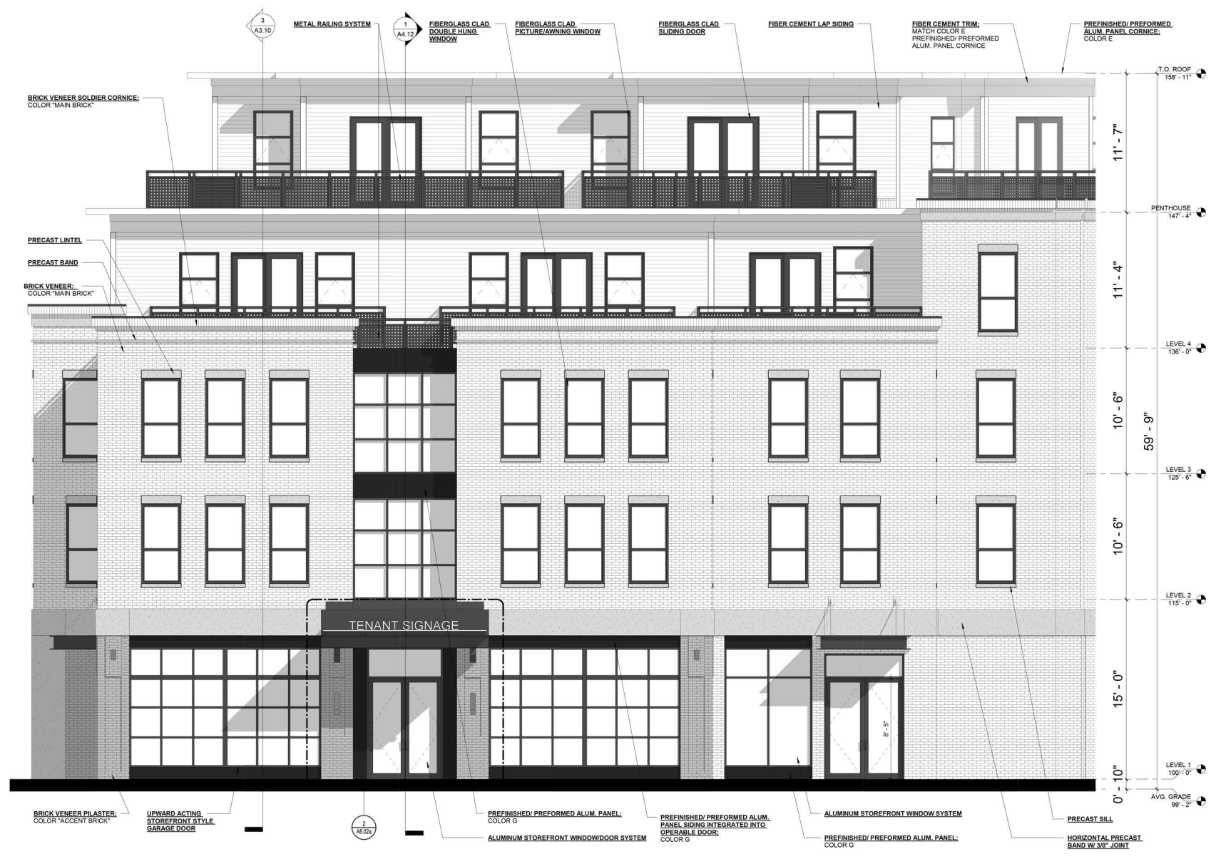
2 EXTERIOR ELEVATION - SOUTH SCALE: 1/4" = 1'-0" REF SHEET: 1 / A1.01
