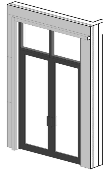
4A ENLARGED STOREFRONT WINDOW/DOOR IN METAL PANEL AT STAIR LEVEL 1 3D SCALE:
