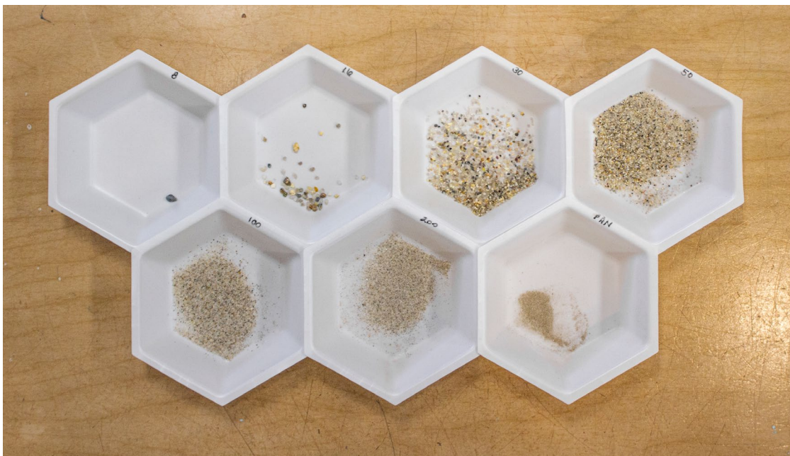
Washed and sieved sands sorted according to sieve size (color corrected fluorescent light)
