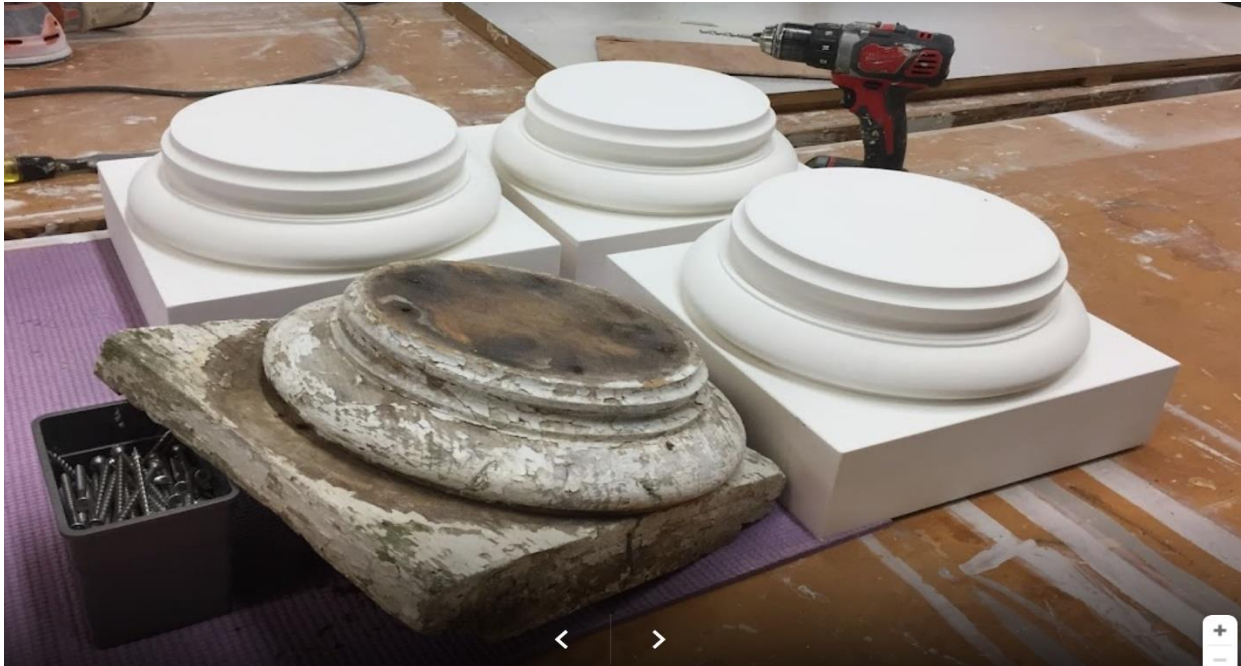
Proposed column and pilaster base construction. This is to only illustrate how the new bases will be made. 1-piece solid PVC
