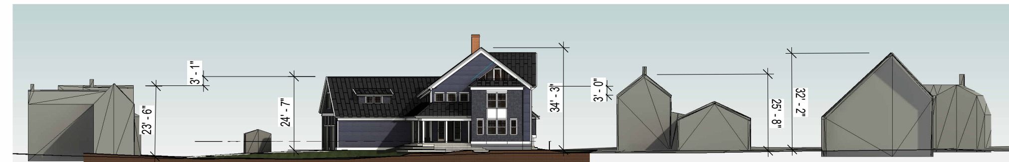
4 EAST ELEVATION - WATER SIDE 1/32" = 1'-0"
