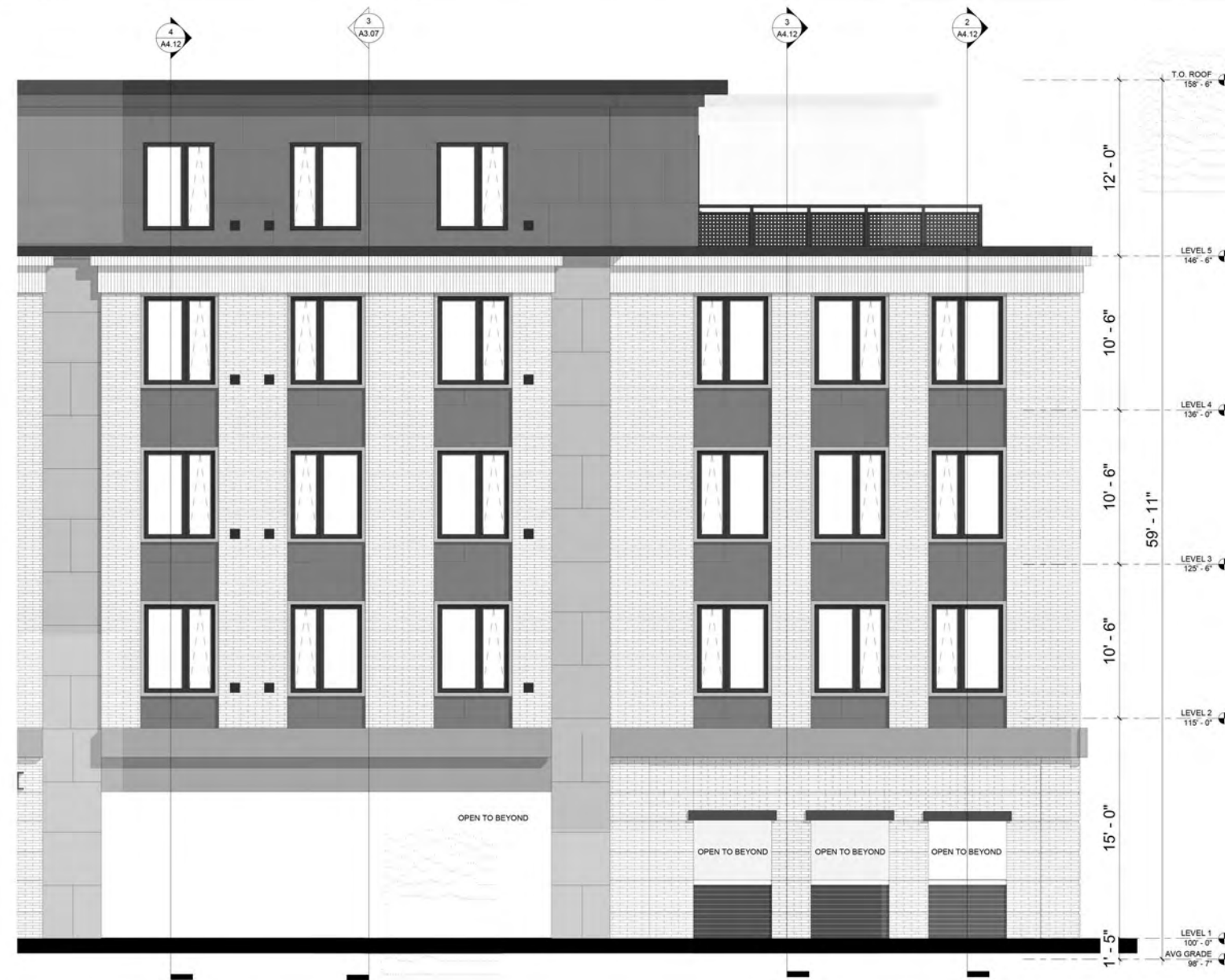
① NORTH EAST ELEVATION A SCALE: 1/4" = 1'-0" REF SHEET: 1 / A1.02
