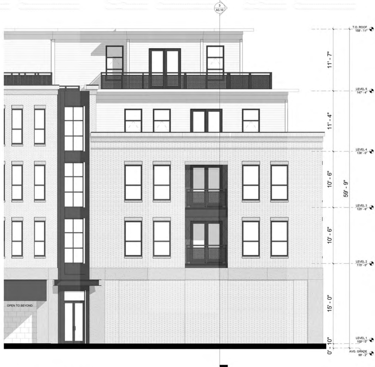
1 EXTERIOR ELEVATION - NORTH SCALE: 1/4" = 1'-0" REF SHEET: 1 / A1.01
