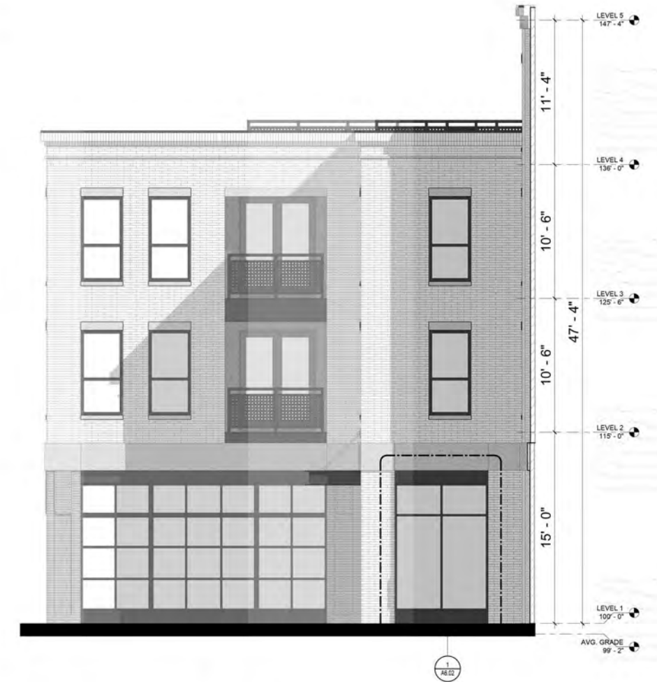
1 EXTERIOR ELEVATION - EAST SCALE: 1/4" = 1'-0" REF SHEET: 1 / A1.01
