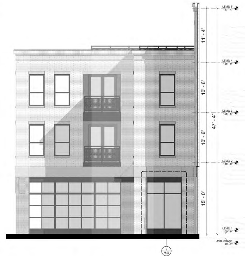
1 EXTERIOR ELEVATION - EAST SCALE: 1/4" = 1'-0" REF SHEET: 1 / A1.01
