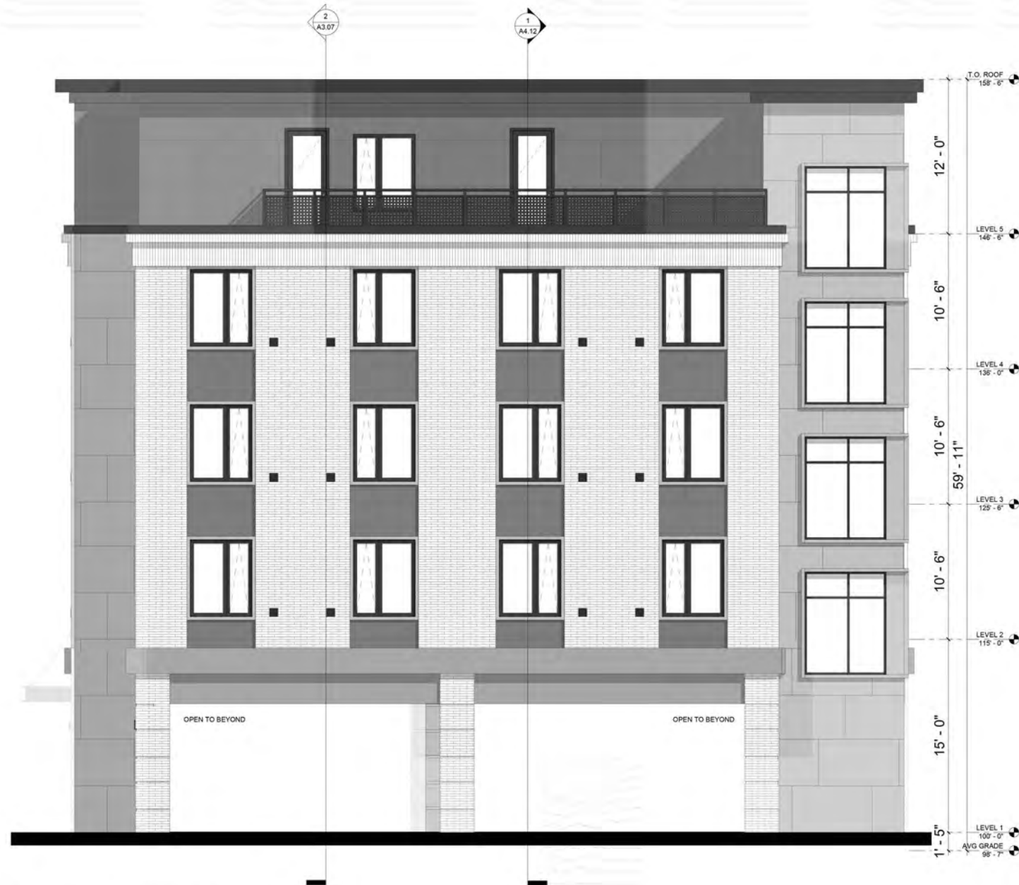
2 NORTH WEST ELEVATION B SCALE: 1/4" = 1'-0" REF SHEET: 1 / A1.02
