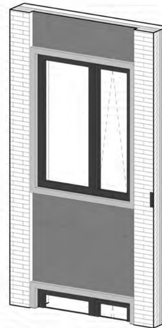
2A ENLARGED VINYL WINDOW IN METAL PANEL/BRICK VENEER L2-4 3D SCALE:
