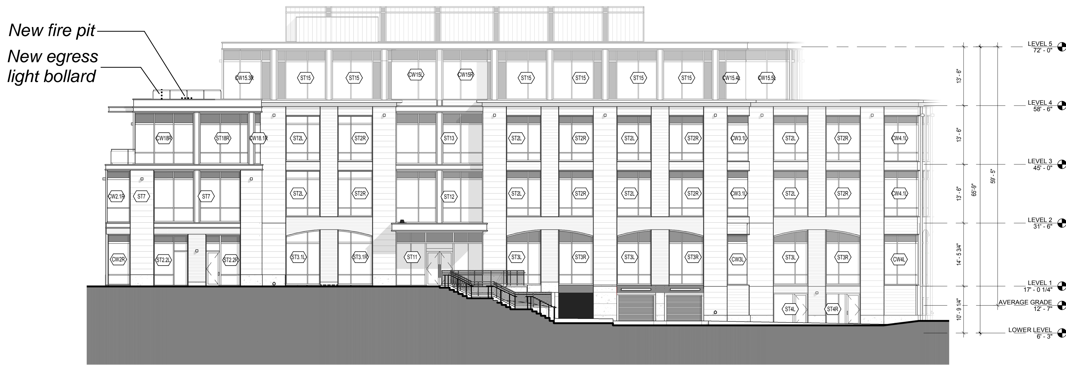
1 HDC BUILDING ELEVATION - ENTRY PASSAGE (EAST) 3/32" = 1'-0"
