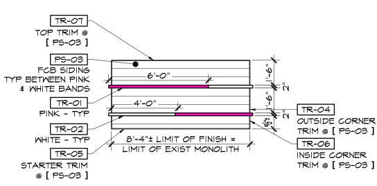
2 D/T MONOLITH DETAIL (A3.1) **SCALE**: 1/4" = 1'-0"
