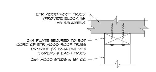
TYP - SOFFIT CONNECTION DETAIL SCALE: 3" = 1'-0"
