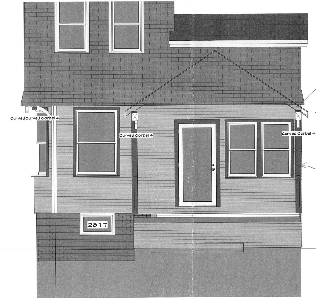
Aspholt Shingks 5/8 Zip Rod 2x8 RAFIERS with 2x6 overlags 6x6 HEADERS CX6 HEADERS Ed Corbel 4 6 x 6 Posts with Applicable FASTNERS Wew winklows tempered glass L 2X8 Joists 16 oc with Hangers AN posts supported by 10" SONNA TUbes with Big Foot
