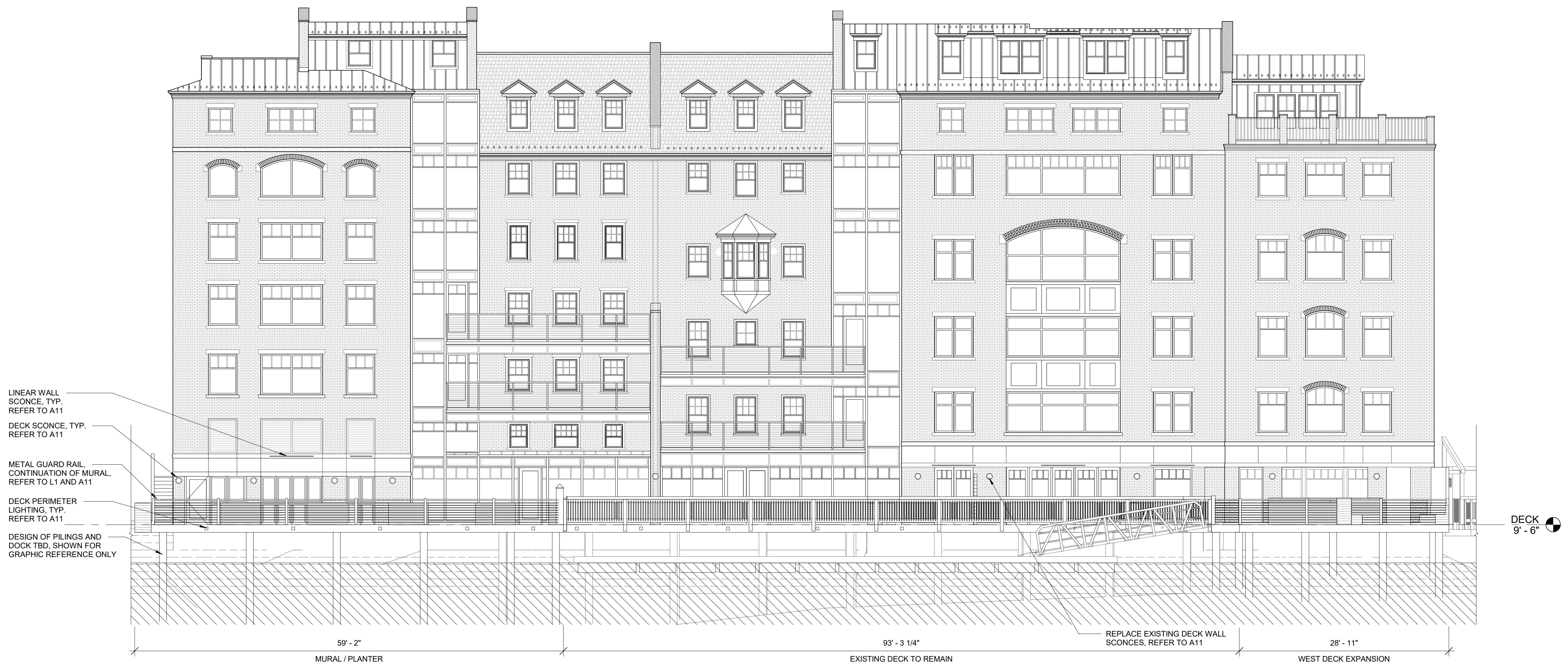
1 PROPOSED NORTH ELEVATION 1/8" = 1'-0"
