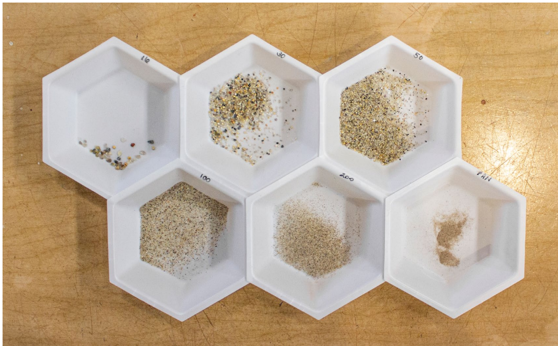
Washed and sieved sands sorted according to sieve size (color corrected fluorescent light)
