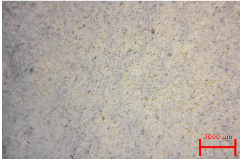
Photomicrograph of the weathered face of the bulk sample before digestion (incident daylight-balanced light, 10x magnification).
