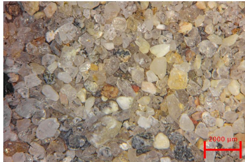
Photomicrograph of the extracted aggregate before sieving, note (incident daylight-balanced light, 10x magnification).
