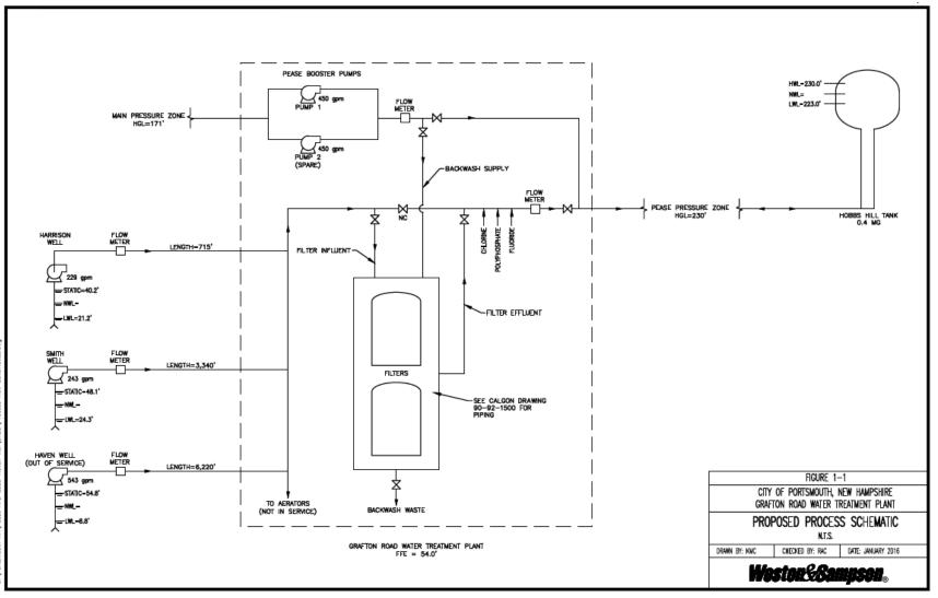
Figure 1-1 – Current Temporary Treatment Process Flow Schematic
