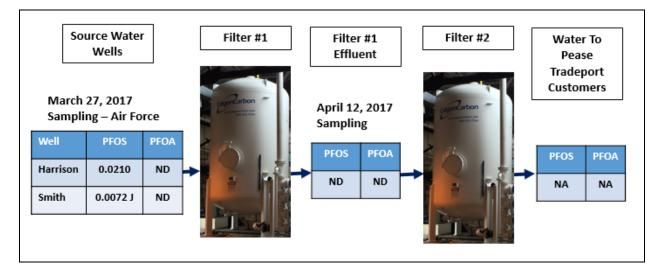
The activated carbon demonstration filters for the Harrison and Smith wells have been on line since mid-September 2016. The City's engineering consultant continues to sample the performance of the filters based on the volume of flow going through the filters. The graphic above shows the most recent source water sampling and treated filter water quality results for the PFOS and PFOA. A summary of the
