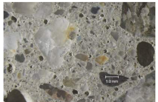
Magnification: 15x Description: Hardened air void system.
