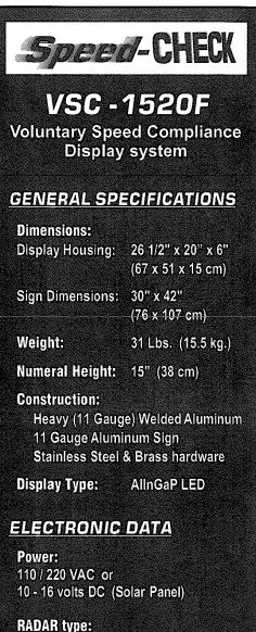
RADAR type: Low power - 24.150 Ghz (K-band)
