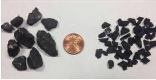
Figure 3-4. Activated carbon media
