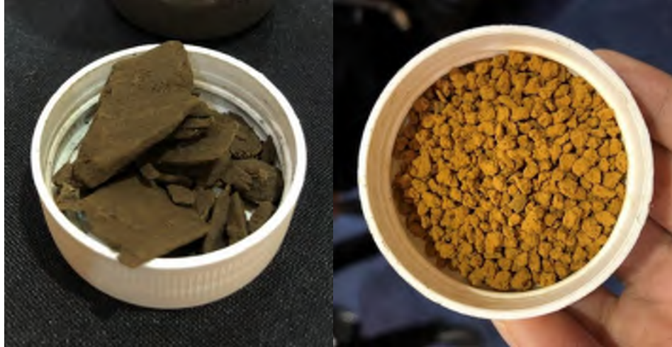
Figure 3-3. Iron sponge media (left) and granular iron hydroxide media (right)
