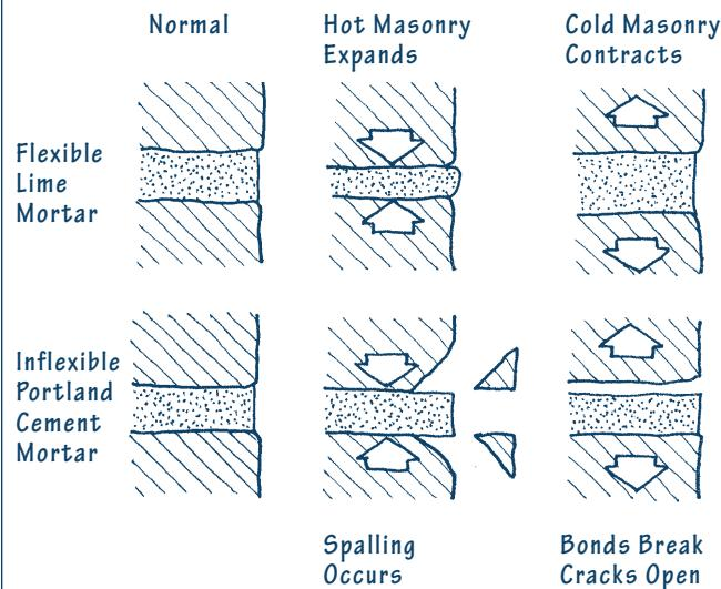
Temperature changes cause masonry units to expand when heated and contract when cold. This expansion and contraction results in compression and flexing of the adjacent mortar joints.
