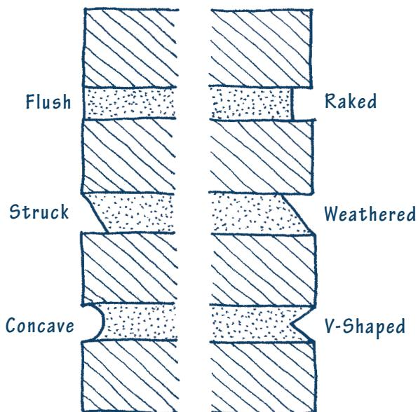
There are numerous mortar joint profile types, or shapes, with each producing different shadow lines and highlights. When repointing an area of masonry, it is important to tool the mortar to match the existing joint profile for a consistent appearance.
